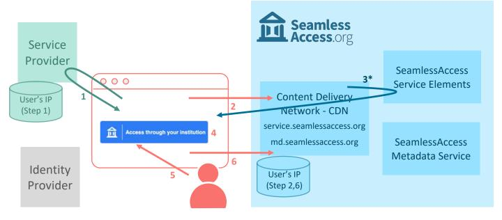
**1.** User accesses the Service Provider's (SP) site, which will likely log user's IP address. In order to render the SeamlessAccess Button, the SP uses the component library provided by SeamlessAccess at **service.seamlessaccess.org/thiss.js**.
